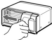
Always use the unit with the door closed. Otherwise, foreign matter may enter the unit and contaminate the lenses inside the changer.
